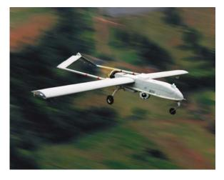
The AAI Shadow 200 UAV with a payload of 27 Kg, a takeoff weight of 170 Kg and an estimated range of 600 Km. Image kindly supplied by <u>www.aaicorp.com</u>.
