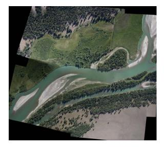
An image of a region in British Columbia, Canada, created by stitching together 160 separate aerial photographs, taken at 2,100 feet altitude, by the CropCam, a small Unmanned Air Vehicle.
