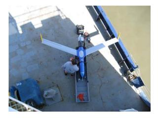
The InSitu / Fugro GeoRanger UAV on a ship. The GeoRanger currently has a fuel and payload capacity of 5.4 Kg, a value that might change with ongoing developmental work. Image kindly supplied by <u>www.insitu.com</u> and <u>www.fugroairborne.com</u>.
