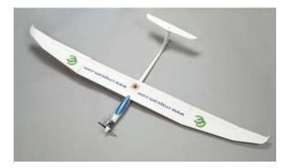
The 8 foot wingspan CropCam Unmanned Air Vehicle used to photograph agricultural and forest lands. Images kindly supplied by <u>www.cropcam.com</u>.
