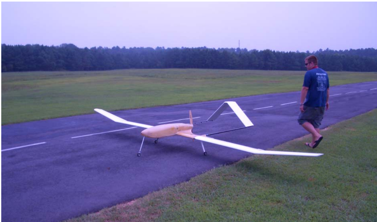
Figure 96 The hydrogen fuel cell powered UAV developed at the Georgia Institute of Technology
