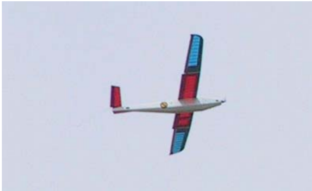
Figure 95 The “Spider-Lion” micro UAV powered by a hydrogen fuel cell
