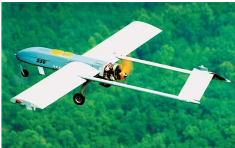
Figure 2 = A Shadow 200 Unmanned Air Vehicle, with “pusher” motor. REF 68
