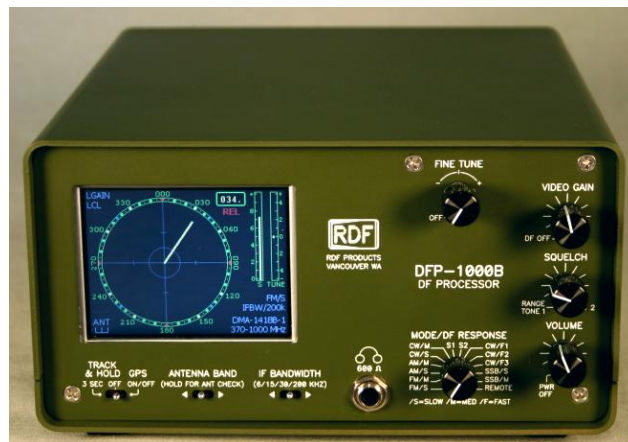
Figure 109 = Example of a Radio Direction Finding device with multiple antennas. REF 38
