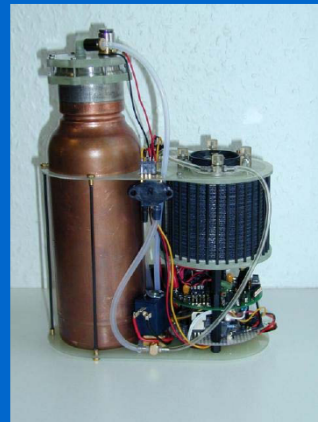
Complete system : 220 Wh/kg energy density 2,27 kg mass system
