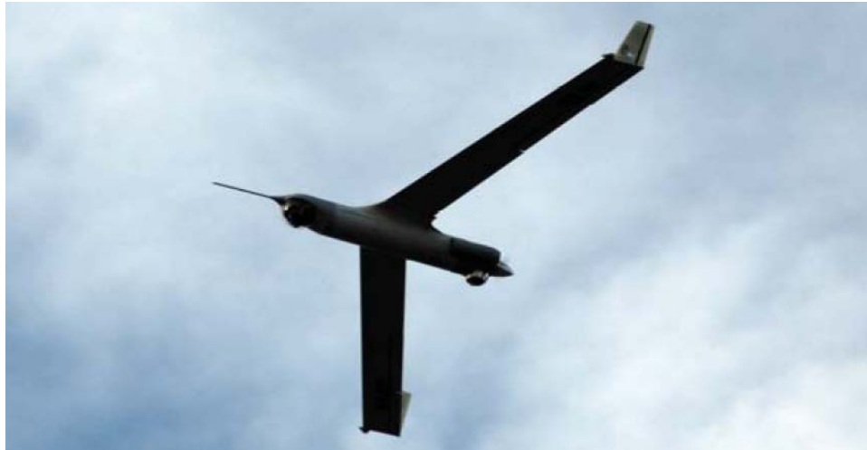
Figure 15 = Notice the absence of a tail fin in this UAV
