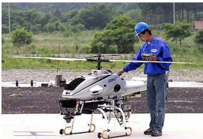
Figure 63 = Getting the unmanned Yamaha RMAX helicopter ready for a test flight. REF 32
