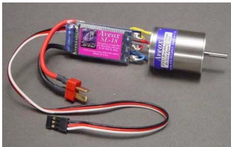
Figure 100 Aveox/Zagi brushless d.c. motor with electronic motor controller http://www.zagi.com/index.php?main_page=aveox_mod
