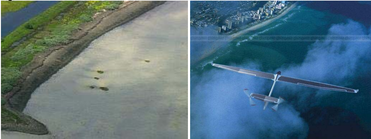
Figure 50 = Solar powered UAVs promise very long endurance times, measured in days. REF 26
