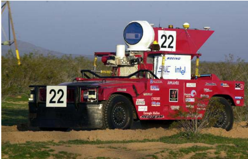
Figure 22 = Carnegie Mellon University “Red Team” best performing, fully autonomous, vehicle in the DARPA Grand Challenge 2004. REF 69
