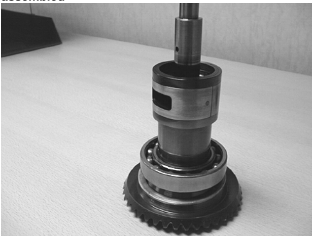
Fig 8. Sprung expanding ring valve seal fully assembled
