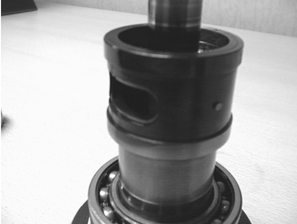
Fig 7. Sprung expanding ring valve seal with sliding seal and compression seal removed.
