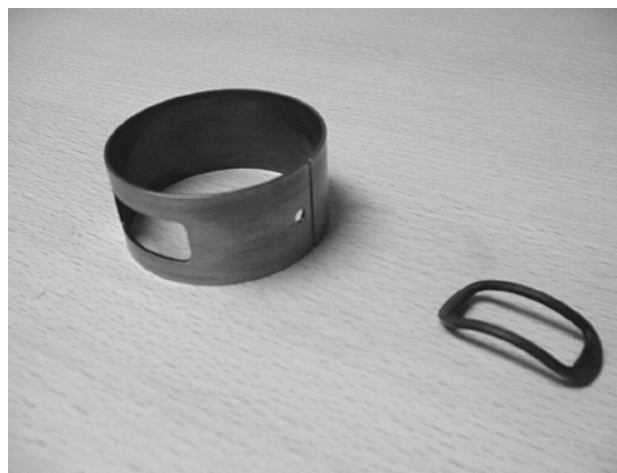
Fig 6. Sprung expanding ring valve sliding seal and compression seal
