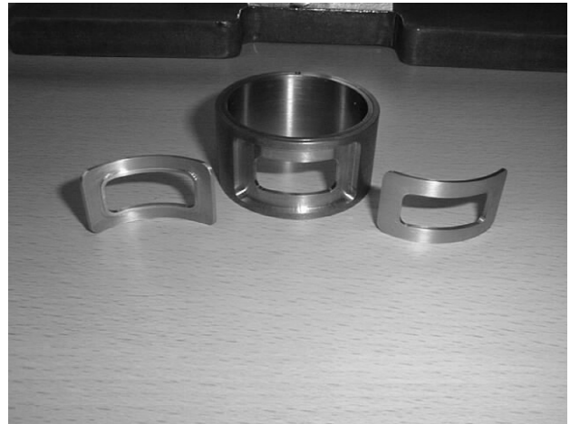
Fig 4. Simple valve seal. Sliding seal rear view, inner and outer sleeves assembled, sliding seal front view.
